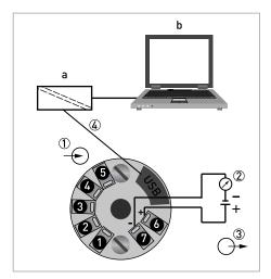
Figure 5-1: Connection during configuration of in-head transmitter
