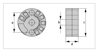
Figure 7-2: In-head transmitter
