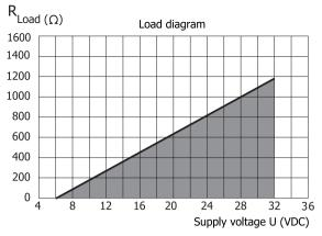
Maximum load depending on power supply Formula for the max. permissible output load for APAQ C130<sup>TC</sup>:
