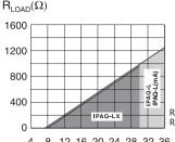
R<sub>LOAD</sub>=(U-7.5)/0.22 IPAQ-L, IPAQ-L(mA)  $R_{LOAD}^{LOAD} = (U-8)/0.22 IPAQ-LX$
