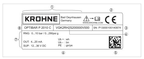
Figure 2-1: Example for nameplate
