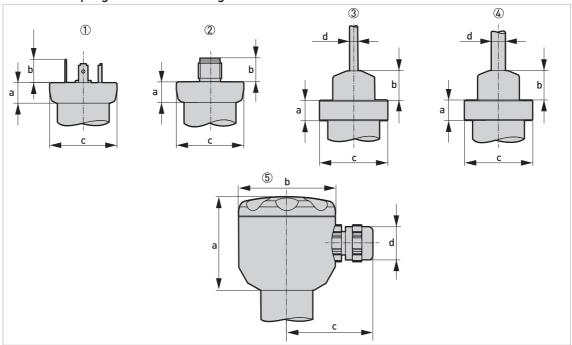
Figure 6-1: Dimensions for connection plug and field housing
